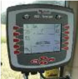
**Computerised spray rate controller:** automatically adjusts spray application rate to forward speed. The Muller system shown also controls boom hydraulics and steering system from either the main screen or joystick (supplied).
