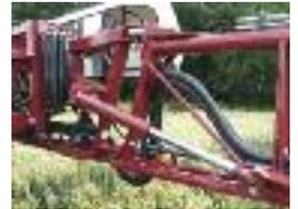
All nozzles and spray lines are secured above the base of the boom for protection against accidental damage.
